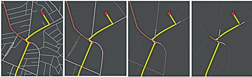
**Figure 2.** One possible application of brain-computer interfaces is adjusting the visual representation of data to fit users' needs or cognitive strengths. This example shows a vehicle GPS system slowly fading noncritical information in and out—in this case, surrounding streets—depending on the driver's workload.
