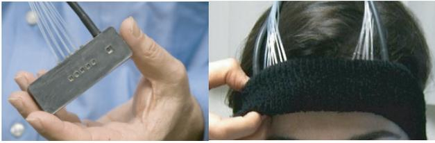
Figure 2: (Left) An fNIRS probe with five light sources and one detector. (Right) A headband holds two fNIRS probes in place on a study participant's forehead.
